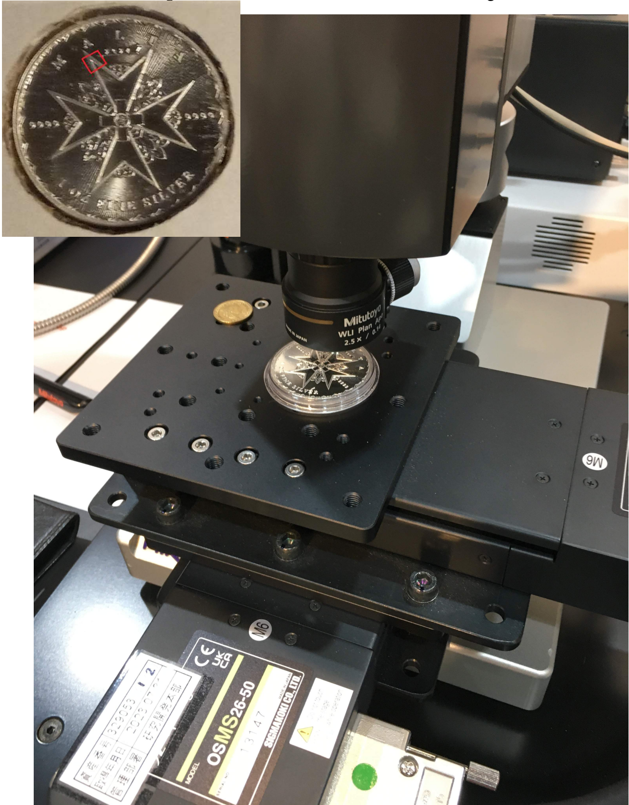
Maltese Cross Bullion under Mitutoyo WLI Unit
